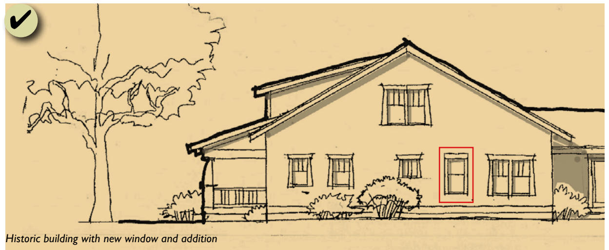
Figure 93: Design a new window opening to match historic window proportions on the same façade. The image above illustrates the historic building. The image below shows an appropriate location for a new window in the historic building.
