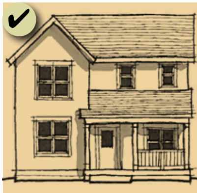
Figure 141: This two-story building is compatible in several contexts. It has a similar roof form, window pattern and porch proportion to historic buildings in the neighborhood.
