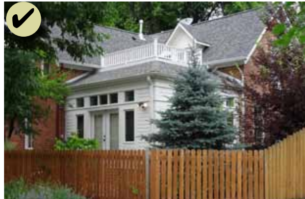
Figure 181: Differentiate an addition from the original structure with an offset and change in material.
