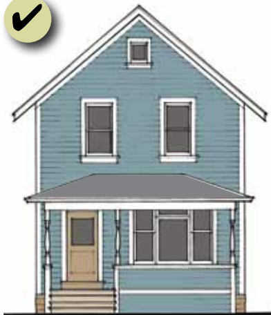
Figure 117: When designing a color scheme, consider the entire composition: The back plane of the main façade is a major surface for which a scheme should be devised. A color scheme for the front plane, composed of a porch in this case, should also be designed.
